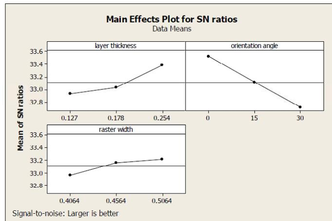
Figure 9: Main Effect Plots for Surface Roughness
